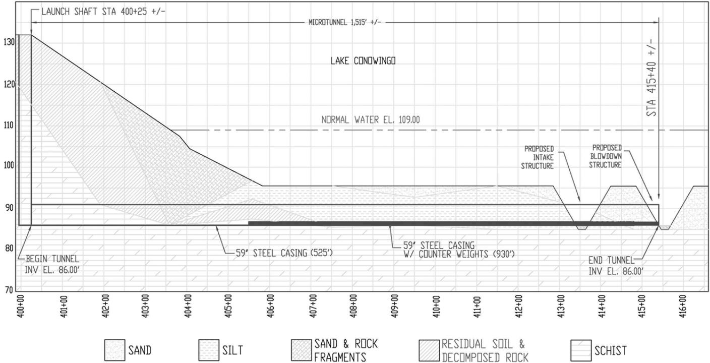
**Figure 5, Final Design – Profile View**
