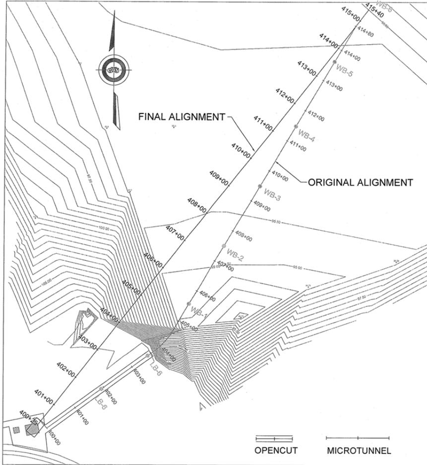
**Figure 6, Final Design – Plan View**
